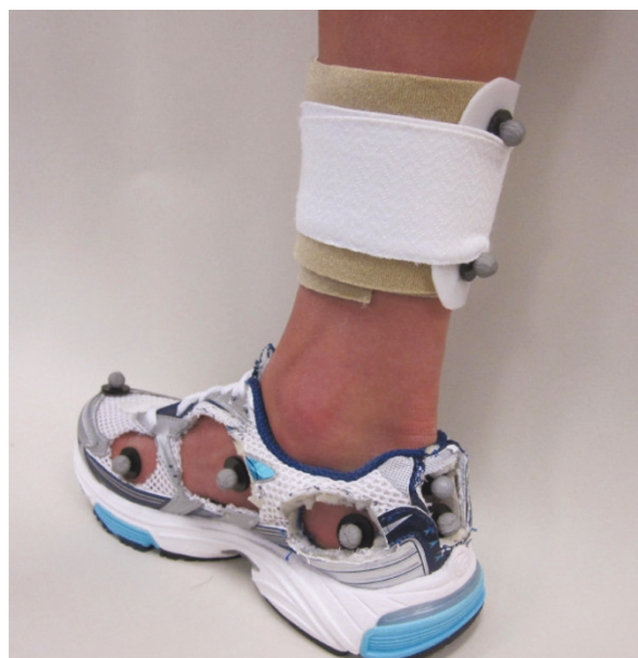
Figure 3 Marker set-up for kinematic data collection.
