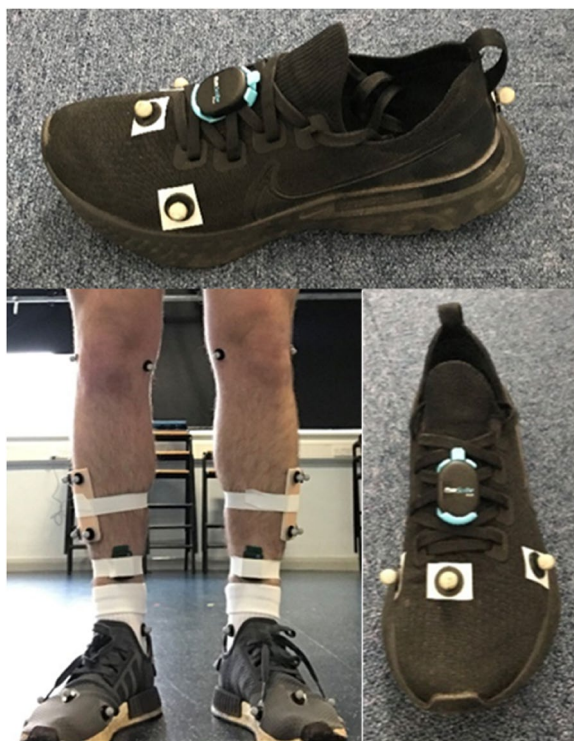
Fig. 1 Marker and equipment placement on lower limbs and participant footwear
